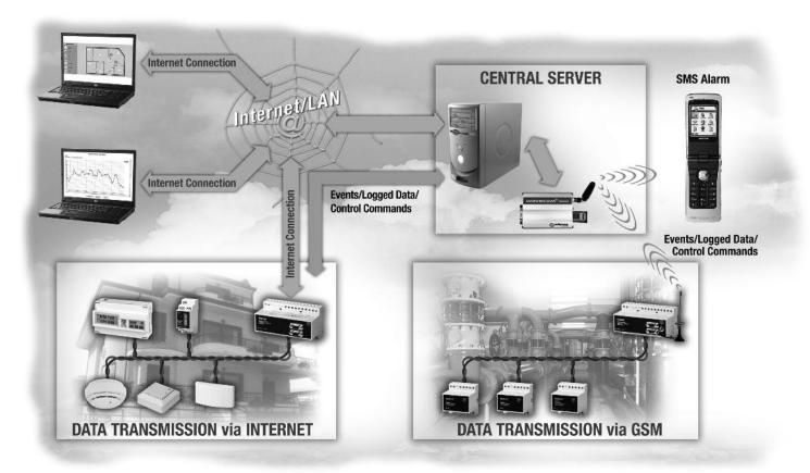
After the Dupline<sup>®</sup> Data Logger has been programmed, it needs to be registered on www.dupline-online.com. In this way the Central dupline-online Server gets the unique ID code of the Data Logger and it gets information about the descriptions and scaling of the data that it will receive from the Data Logger via the Internet or the GSM network. During registration, the user also gets a user name and password (unless the Data Logger is registered under an existing user name).
